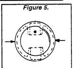
3. Check wrist Pin for Looseness:- A rough check for wear in the wrist pin, wrist pin bore in the piston, or wrist pin bore in the connecting rod is to check for looseness or play with the piston assembled to the rod. Looseness or play indicates a worn wrist pin, or a worn bore in the piston or connecting rod.
